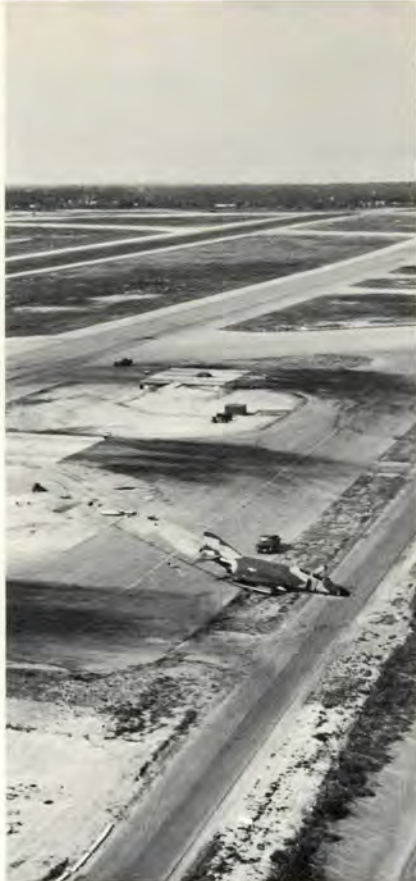
Blown tire from wheel striking barrier tape guide resulted in F-4 mishap. Compare photos above. Note edge striping, location of lights.
