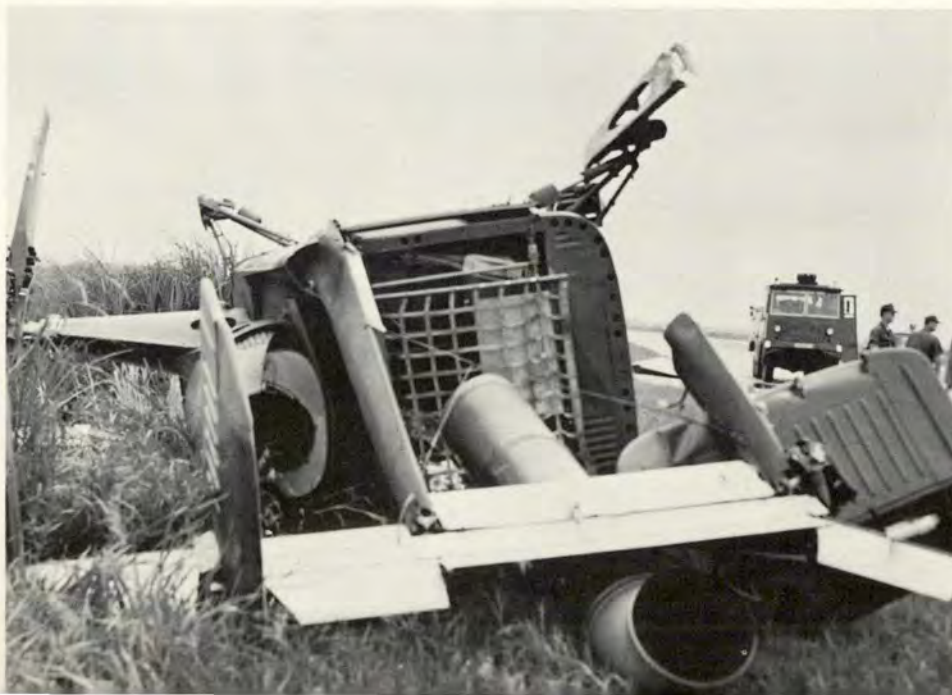
Bent bearpaw is silhouetted against sky in this photo of wrecked HH-43 helicopter. Bearpaw caught on cable when aircraft rolled over BAK-9.
