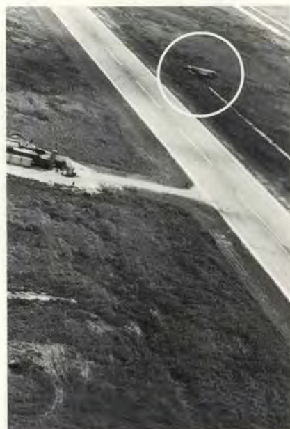
There's always a ditch. Damage would have been light if ditch hadn't interrupted this C-47 which left the runway after pilots lost control.
